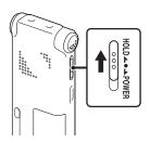
Slide the HOLD/POWER switch in the direction of "HOLD."
